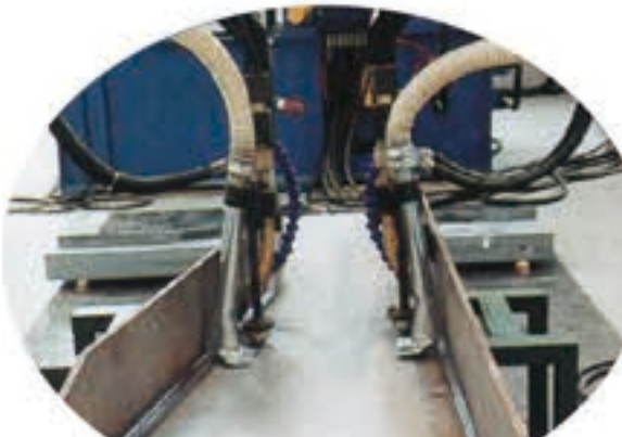
变截面H型钢的焊接 Welding of the Variable Section Beam
