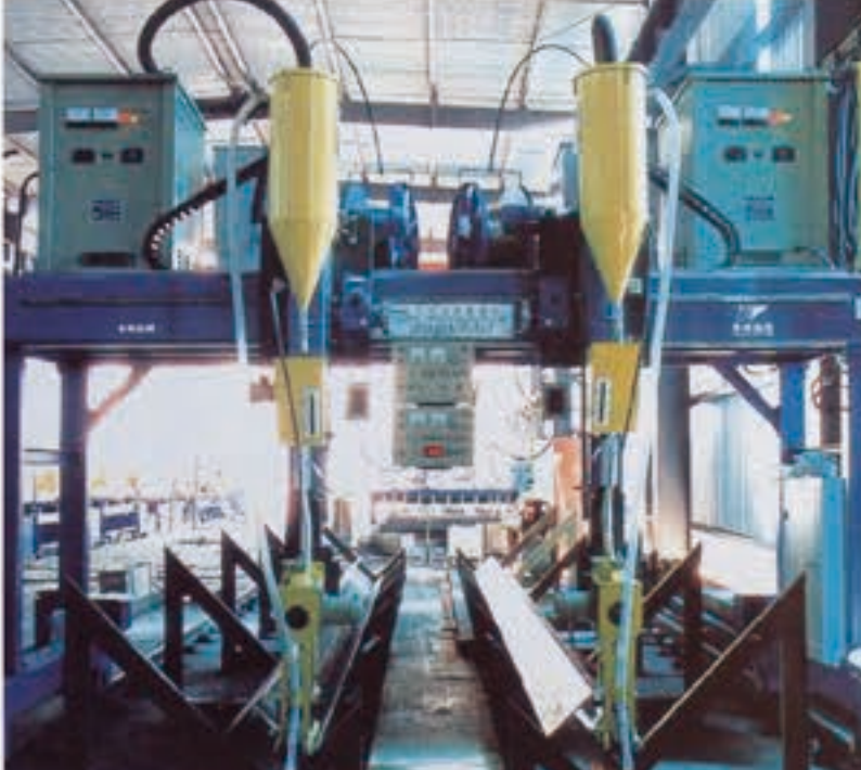
集中控制的龙门焊 Centrally-controlled gantry Welding
