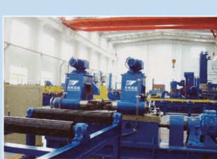
HYJ-600 H型钢翼缘矫正机 HYJ-600 H-beam Flange Straightening Machine
