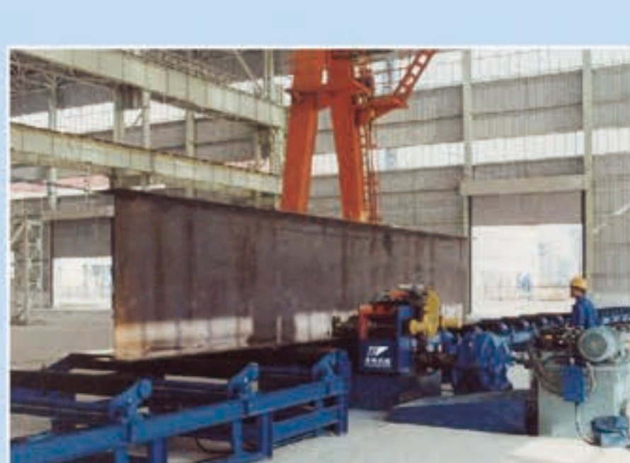
YJB-608液压矫正机 YJB-608 Hydraulic Straightening Machine
