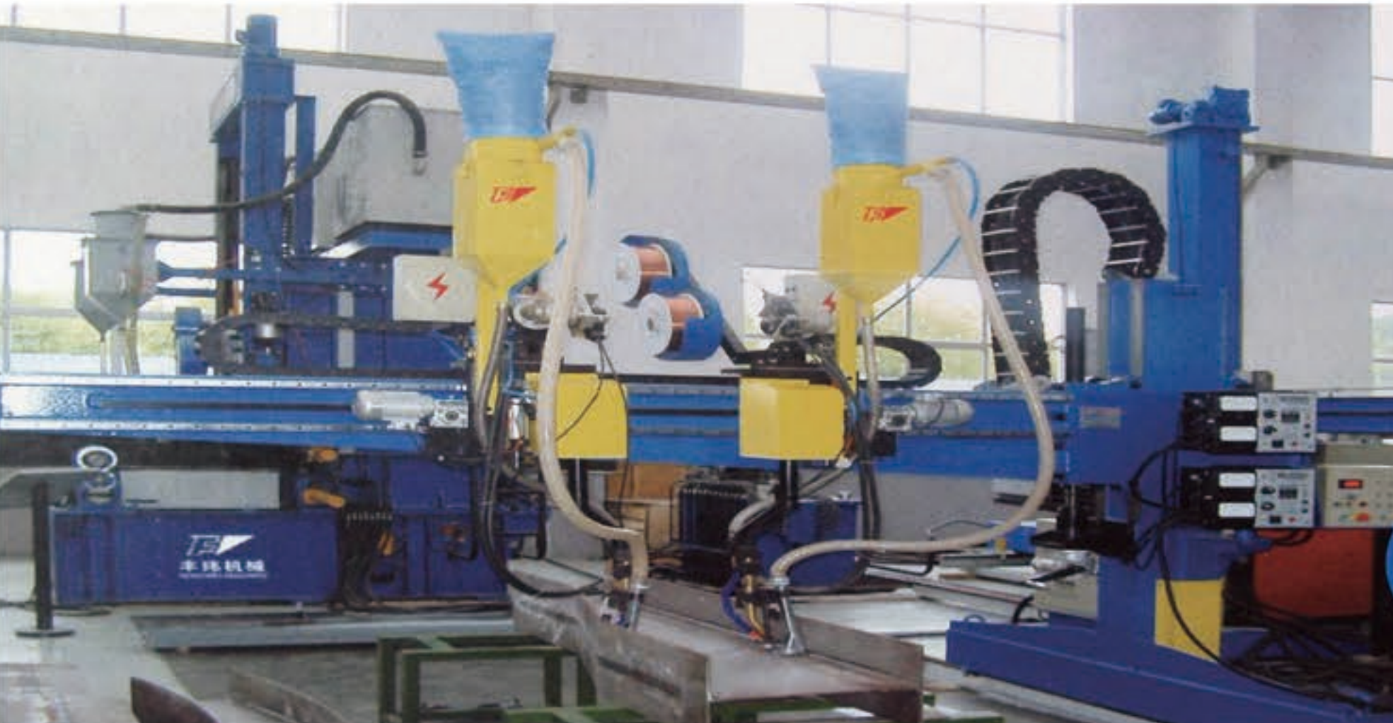
变截面H型钢焊接机 Variable Section H-beam Steel Welding Machine
